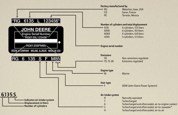
\*S engines can be modified to be turbocharged and aftercooled, air-to-engine coolant, in dual-circuit keel-cooled applications. Contact your John Deere engine distributor.
