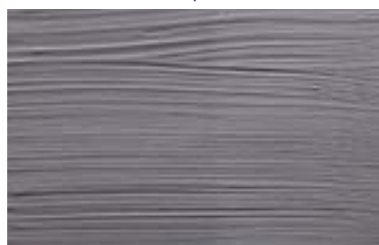
Poor flow properties = uneven film thickness – valleys between brush marks
